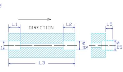
All feedscrews bored 31.75mm (1.2502 inches) and fitted with SSTL tube through
